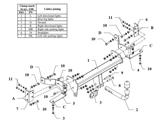
This towing hitch is designed to assembly in following cars: **OPEL ANTARA (C105)**, produced since 2006, catalogue number **E51** and is prepared to tow trailers max total weight up to **2000 kg** and max vertical mass **80 kg**.
