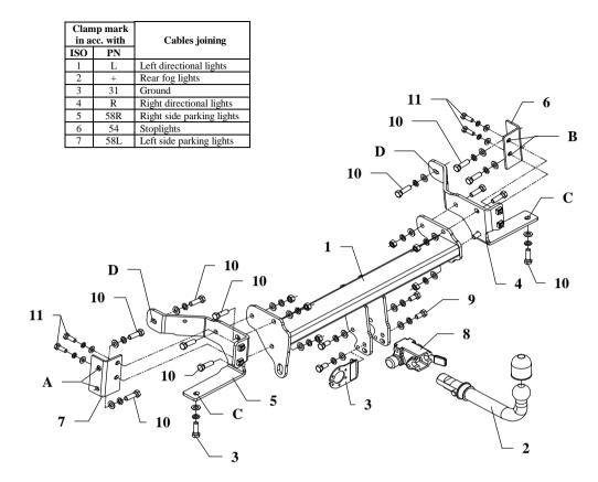
This towing hitch is designed to assembly in following cars: **OPEL ANTARA (C105)**, produced since 2006, catalogue number **E51A** and is prepared to tow trailers max total weight up to **2000 kg** and max vertical mass **80 kg**.
